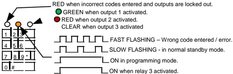
To activate your gates or door via keypad, simply enter the 4 digit code which has been programmed by your installer.
